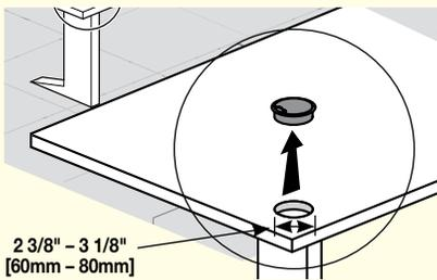
2. Put edge guard in place and feed up data cable.
