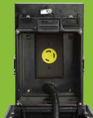
30 amp, 250V Turnlok® locking receptacle L6-30R
