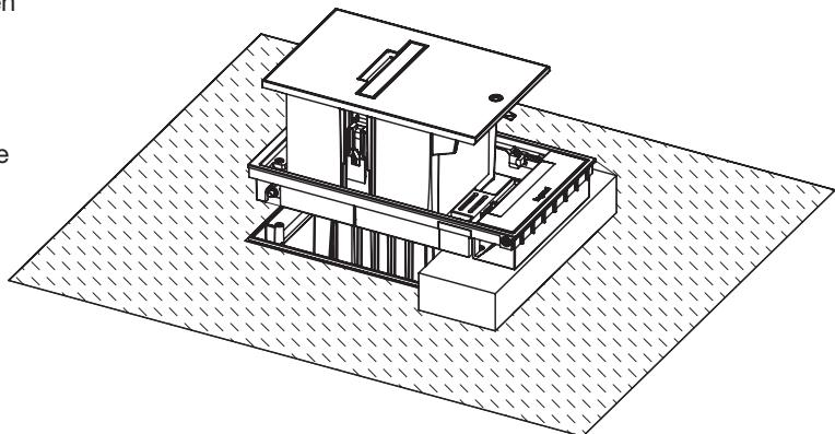
**4** Using a 9/64 hex key (not supplied) remove the (2) screws holding the door to the flange. Remove the door taking note of the orientation of the springs positioned on either end of the door.
