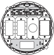
\*68DB mounting plate is required for all 68 device plates.
