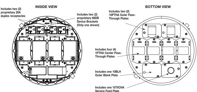
NOTE: For more information on Device Plates and Bottom Feed Plates and on the additional options available, see the Device Plates and Bottom Feed Plates sections found later in this document.
