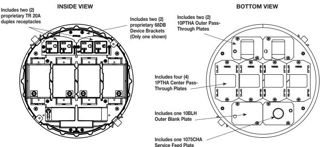
NOTE: For more information on Device Plates and Bottom Feed Plates and on the additional options available, see the Device Plates and Bottom Feed Plates sections found later in this document.
