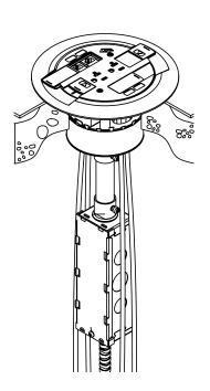
**Step 15.** Push Poke-Thru unit into concrete to complete installation.
