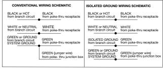
WARNING: Ground wire from junction box must be connected to SYSTEM GROUND.
