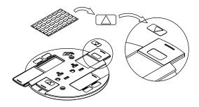
**NOTE:** The orange triangle shall only be placed on devices that are wired for isolated ground. See NEC 250-146(d).
