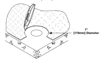
For Tile Applications up to a Maximum of 3/4" [19.1mm] Thick.
