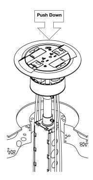
CAUTION: Poke-Thru cannot be rotated in hole after insertion into floor.
