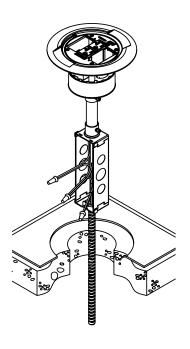
**Step 8.** Connect Poke-Thru conductors according to required device configuration. See schematic below.
