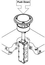
**CAUTION**: Poke-Thru cannot be rotated in hole after insertion into floor.
