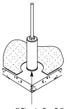
4" Diameter Core Drill 4 1/16" [103mm] Actual Diameter
