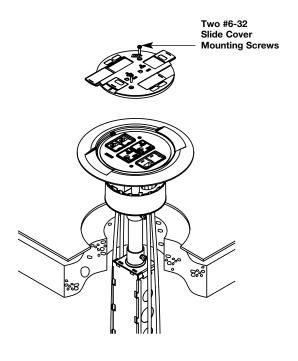
**CAUTION:** Do not over tighten cover mounting screws.
