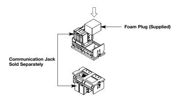
CAUTION: Empty communication ports must be closed off with foam plugs or TracJack blanks to maintain fire classification.
