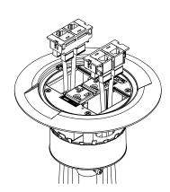
Step 13. Align gasket over receptacle and press bead into flange channel.
