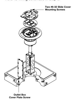
Step 7. Wire the power circuit.
