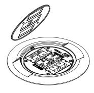
**CAUTION:** Gasket must be set in place to provide scrub water seal.
