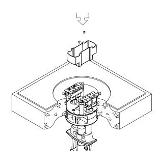
**Step 8.** Feed communication jacks through the trim flange and snap into place. Attach trim flange to stem assembly with the four #6-32 screws provided
