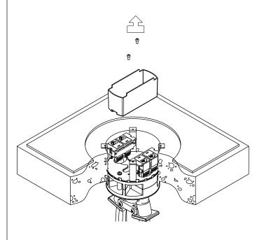
NOTE: Make sure that the carpet cutout is a 7" [177mm] dia. cutout. If the carpet cutout is not 7" [177mm] diameter, use template which is provided on the back of this instruction sheet to make the correct opening in the carpet.
