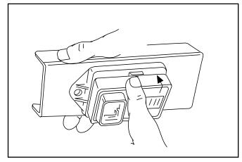
3. Select adapter cover to be used, snap adapter into AMTPN/25DTPN wire per instructions. Snap AMTPN/25DTPN to space provided at bottom of pole.
