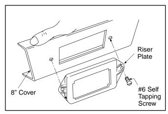
2. Screw riser plate into 8" cover section provided, using #6 self tapping screws.
