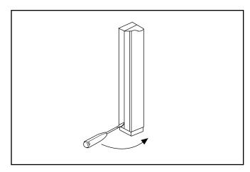
Insert screw driver into slot, turn slowly, adjust pressure.
