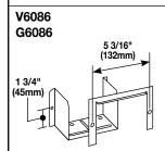
Panel Connector – For connecting 6000 with surface type panel boxes. Accommodates maximum wire capacity of 6000 system. Separate C-flange fits around raceway, covering uneven cuts to the box. Cut 4 3/4" x 3 9/16" (121mm x 90mm) hole in panel box.
