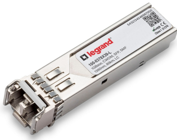
Calix 100-0378X39 Compatible 1000Base-CWDM SFP Transceiver (SMF, 1390nm, 80km, LC Duplex, DDM, I-Temp)
