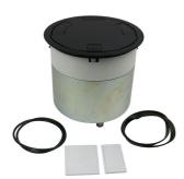
For use with 10" (254mm) diameter hole. All devices are recessed 4 1/2" (114mm) below the finished floor level. Unit ships complete with an all aluminum cover (assembled) designed to sit on top of finished floor surface (carpet, tile, wood, concrete or terrazzo). Covers are available in the following powder coated finishes: black (BK), gray (GY), nickel (NK), brass (BS) and aluminum (AL).
