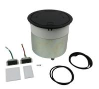
For use with 10" (254mm) diameter hole. Cover and stem are pre-assembled together. All devices are recessed 4 1/2" (114mm) below the finished floor level. Unit ships complete with an all aluminum cover (assembled) designed to sit on top of finished floor surface (carpet, tile, wood, concrete or terrazzo). Covers are available in the following powder coated finishes: black (BK), gray (GY), nickel (NK), brass (BS) and aluminum (AL).
