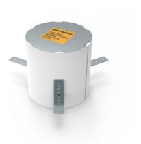
The Pre-Pour sleeve allows contractors to plan where a poke-thru device will be placed in the construction process. This eliminates the need for costly core drilling.
