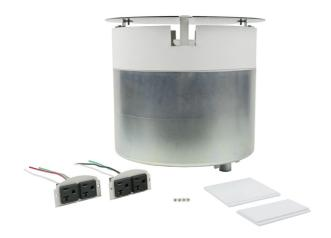
For use with 10" (254mm) diameter hole. All devices are recessed 4 1/2" (114mm) below the finished floor level. Unit ships complete with a disposable construction cover. Unit works with 10" Evolution cover assemblies (10CTC). All cover assemblies are sold separately and are available in the following finishes: black (BK), gray (GY), nickel (NK), brass (BS) and aluminum (AL).
