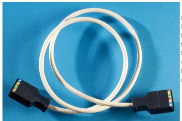
Clarity 110 patch cords are ETL verified to TIA-568-B Category 6 and 5e component standards. More importantly, Clarity 110 plugs utilize an internal signal feedback technique to control cross talk without compromising impedance. Clarity 110 to modular 8 position patch cords utilize both signal feedback and center tuning. This allows more transparent connector interfaces for significant elevation of channel performance that can be field measured.
