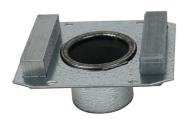
Two-gang 1 1/2" trade size conduit housing assembly. Use on 8AT, 8ATC, and 8STC Series Devices. Covers two available center compartments. Both compartments will be the same service.
