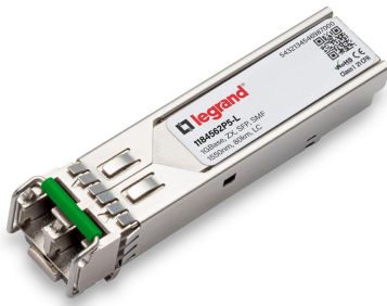
Adtran 1184562P5 Compatible 1000Base-ZX SFP Transceiver (SMF, 1550nm, 80km, LC Duplex, DDM, I-Temp)
