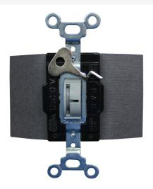
Locking Manual Controller, Single-Pole, Double-Throw Switch. 15A, 120/277VAC rating, Tested to 3A, 24VDC rating.
