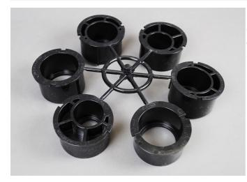
Conduit reducing ring allows for 1 1/4" conduit hub (for RPNFB only) to allow for smaller conduit feeds where needed. Ring includes: two (2) blanking plugs, (2) 3/4" trade size plugs, and (2) 1" trade size plugs.
