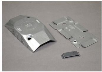
Base and cover each have 1/2"" trade size KO. May be used as a cross, tee, straight through or to terminate run. Two 1500WC Wire Clips included.
