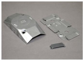
Base and cover each have 1/2"" trade size KO. May be used as a cross, tee, straight through or to terminate run. Two 1500WC Wire Clips included.
