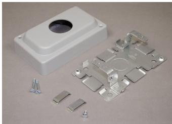
Will accommodate commercially available straight blade and locking single receptacles with face diameters of 1.38-1.40" (35-36mm). Base has 1/2" and 3/4" trade size concentric KOs.
