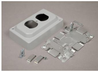
Will accommodate commercially available 15A or 20A duplex receptacles. Base has 1/2" and 3/4" concentric trade size KOs. Nonmetallic cover has 1500 and 2600 Series Raceway twistouts on all four sides. Two 1500WC Wire Clips included. Side wiring recommended. Gray finish. NOTE: Certified to Canadian Safety Standards. For sale in Canada. When ordering these products, add "C" prefix to part number to denote the Canadian version, i.e "C1546B".
