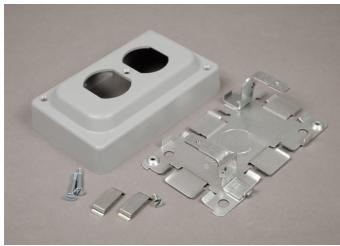
Will accommodate commercially available 15A or 20A duplex receptacles. Base has 1/2" and 3/4" concentric trade size KOs. Nonmetallic cover has 1500 and 2600 Series Raceway twistouts on all four sides. Two 1500WC Wire Clips included. Side wiring recommended. Gray finish. NOTE: Certified to Canadian Safety Standards. For sale in Canada. When ordering these products, add "C" prefix to part number to denote the Canadian version, i.e "C1546B".
