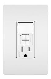
Conducts an automatic test every three seconds, ensuring it's always ready to protect. If the device fails the test, the indicator light flashes to signal that the GFCI should be replaced. It also has our proven SafeLock Protection feature: if critical components are damaged and protection is lost, power to the receptacle is disconnected.
