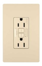
Conducts an automatic test every three seconds, ensuring it's always ready to protect. If the device fails the test, the indicator light flashes to signal that the GFCI should be replaced. It also has our proven SafeLock&trade- Protection feature: if critical components are damaged and protection is lost, power to the receptacle is disconnected.For detailed Tamper-Resistant receptacle information, visit our <u>Tamper-Resistant Receptacles page</u>.
