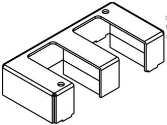
One and a half-gang pass through housing assembly. Used for furniture feed applications on the center compartment only. Only for use with the 6AT Series units.
