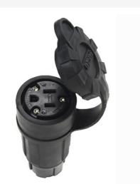
Rated watertight for 1,500 psi high-pressure hosedown, Pass and Seymour watertight plugs and connectors feature multiple seals to ensure protection against the environment. Thermoplastic elastomer (TPV) construction stands up to impacts, oils, chemicals, heat and weather.
