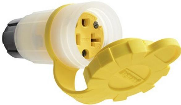
Rated watertight for 1,500 psi high-pressure hosedown, Pass and Seymour watertight GCM plugs and connectors feature multiple seals to ensure protection against the environment. The transparent body houses dual LED lights with 360 visibility, indicating ground continuity and power status, while providing a NEMA 6P/IP67 rating.
