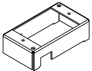
One-gang bottom housing assembly. Designed to accept 175CHA, 175CHA-LJB, 1125CHA, 1PTHA, and 1BLH plates.
