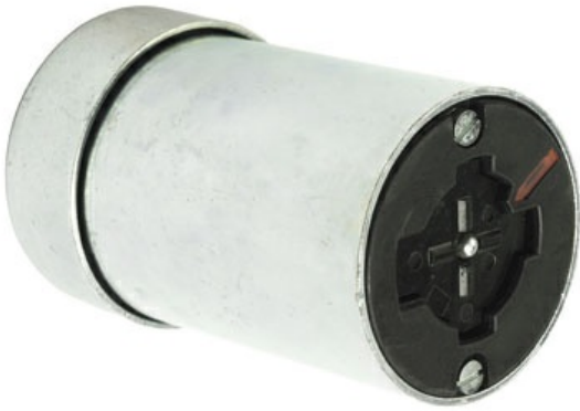
Power Interrupting Connector, Metallic with Rubber Cord Grip 3-Pole, 4W, 30A/600V, 20A/250VDC, 0.36-0.48 ARM
