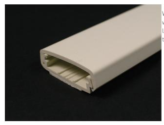
Wiremold 2300 Series Raceway is a low-profile, two-piece raceway with durable, textured PVC ivory finish. Available in 5' (1.52m) lengths. Packed 50' (1.5sm) per carton. Supplied with wide adhesive tape along its entire length.
