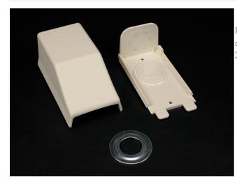
For connecting 2300 Raceway with 1/2'', 3/4'', or 1'' trade size conduit or armored cable. 1/2'' and 3/4'' trade size KO on end, 1/2'', 3/4'' and 1'' trade size KOs on bottom.
