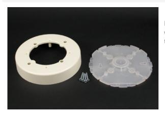
For hanging fixtures, smoke/fire alarms and other security devices with 3 1/2" (89mm) or 4 1/16" (103mm) mounting centers. Has 1/2" trade size KO. Not for use with fans.
