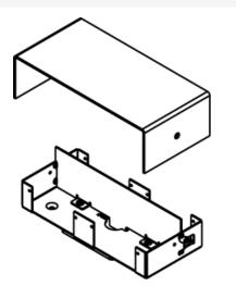
Double width housing for 241 Series Service Head. Barrier included (may not be needed for single service applications). Base has a 3/4" trade size KO for connection to FIT insert. Order two faceplates to complete service head assembly. NOTE: Assembled with scrub water gasket. For use on tile and carpte floors.
