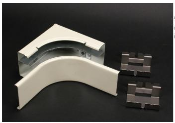
90 degree, divided internal corner elbow provides 2'' (51mm) cable bend radius control for fiber optic and UTP/STP cable installations. Two couplings included.
