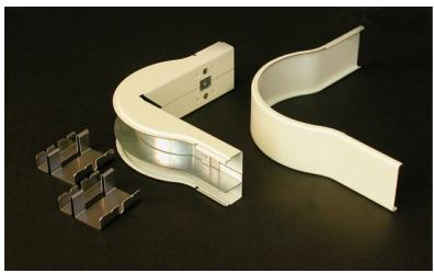
90 degree, divided external elbow provides 2'' (51mm) cable bend radius control for fiber optic and UTP/STP cable installations. Two couplings included.
