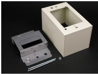
One-gang, labor-saving, over-the-raceway box. Cover has twistout on each side for 2400 Series Raceway. Accepts industry standard faceplates for electrical and communication devices. NOTE: Accepts NEMA single-gang standard faceplates. Certified to Canadian Safety Standards for sale in Canada. When ordering this product for Canada, add "C" to the beginning of the part number to denote Canadian versions, i.e. "CV2444" or "C2444-FW".
