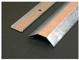
Cover: .050" galvanized steel. Base: .040" (1.0mm) galvanized steel. Packed five 10' (3m) lengths per carton. Base has 9/32" (7.1mm) diameter mounting holes on centers of approximately 8" (203mm).
