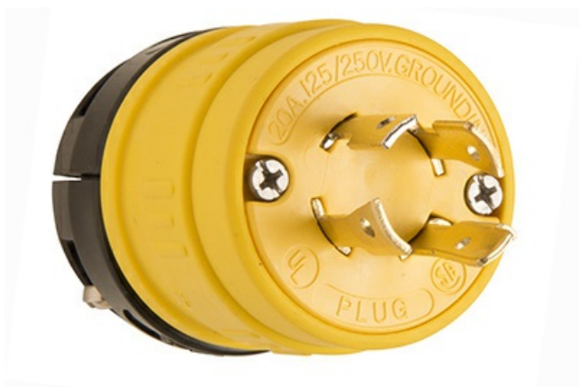
Locking Dust-Tight Rubber Plug, 20amp 125/250volt, NEMA Configuration L14-20
