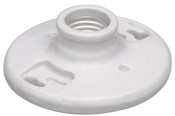
Medium base, porcelain, one piece keyless. 2 terminals with Tamper-Resistant-drive screws, fits 3 1/4-inch and 4-inch boxes, with cage neck.
