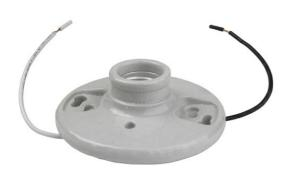
Medium base, porcelain, one piece keyless. 2 terminals with Tamper-Resistant-drive scews, fits 3 1/4-inch and 4-inch boxes, with cage necks, 6-inch Leads.
