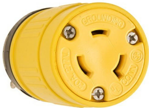
Locking Dust-Tight Rubber Connector, 20amp 277volt, NEMA Configuration L7-20.
