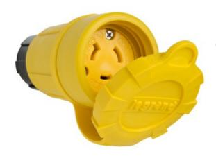
Locking Watertight Connector, 20amp 277volt, NEMA Configuration L7-20, multipoint sealing system provides environmental protection of NEMA 4, 4X, 6, 6P, and IP67 rated.
