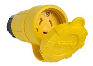
Locking Watertight Connector, 20amp 277volt, NEMA Configuration L7-20, multipoint sealing system provides environmental protection of NEMA 4, 4X, 6, 6P, and IP67 rated.
