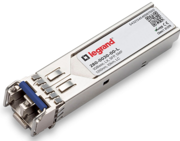
Cyan 280-0030-00 Compatible 1000Base-LX SFP Transceiver (SMF, 1310nm, 10km, LC Duplex, DDM, I-Temp)
