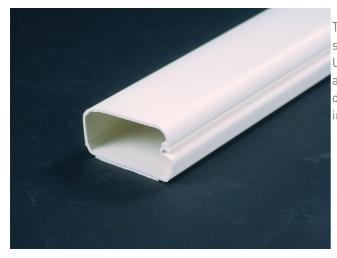
The Uniduct Nonmetallic Latching Raceway System is a one-piece, single channel design, ideally suited to route and protect fiber optic, UTP, and other low-voltage (50V or less) cables in an easy to install and aesthetically pleasing application. 2900 Series Co-extruded design has a smooth plastic finish with adhesive backing. Available in 8ft (2.44m) lengths, packed 160ft (48.8m) per carton.
