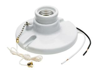
Medium base, porcelain, pullchain, 2 terminals with Tamper-Resistant-drive screws, 6-inch leads, fits 3 1/4-inch and 4-inch boxes with cage neck.
