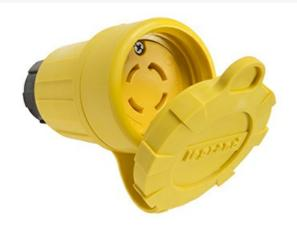
Watertight Connector, 30amp 3Y 120/208V, Non-NEMA Configuration, multipoint sealing system provides environmental protection of NEMA 4, 4X, 6, 6P, and IP67 rated.
