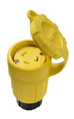
Locking Watertight Connector, 30amp 125volt, NEMA Configuration L5-30, multipoint sealing system provides environmental protection of NEMA 4, 4X, 6, 6P, and IP67 rated.
