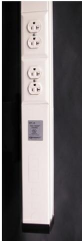
Two-compartment pole (one power, one communication with cross over below power devices). Nominal material thickness .040" (1.0mm). Length 12'5" (3.8m). Two 20A 125V duplex receptacles. One Ortronics Series II adapter. One Ortronics Series II dual Cat 5e insert, two blank inserts and labeling supplies. Maximum ceiling height 10'5" (3.2m).
