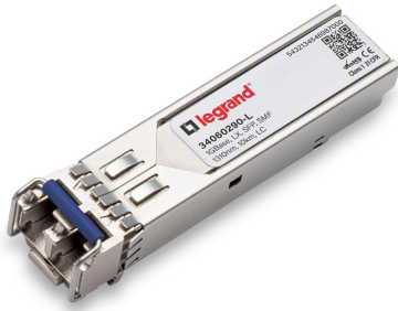
Huawei 34060290 Compatible 1000Base-LX SFP Transceiver (SMF, 1310nm, 10km, LC Duplex, DDM, I-Temp)
