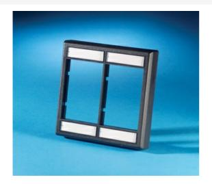
Legrand offers single and double gang Series II plastic Face Plates with a variety of module capacities to match your workstation applications. Series II plates offer recessed label fields, slotted screw holes to adjust alignment and are ruggedly constructed from high impact thermo-plastic 94V-0 rated to ensure long life.
