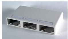
Ortronics Series II Surface Mount Outlet Boxes accept front-loading Series II modules and provide snap-on covers and snap-in label fields. Boxes are supplied with screws and double-sided adhesive tape for mounting onto almost any surface. Compatible with Wiremold 2700, 2800 and 2900 raceway series.
